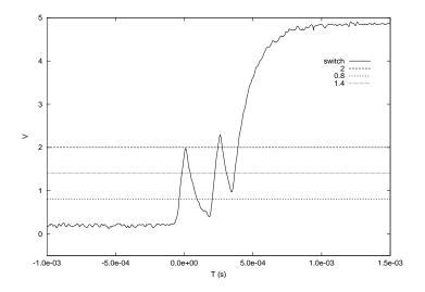
You will need to write an assembly language subroutine that will be called whenever a change of the switch's value is first observed. Your subroutine should delay the processor long enough to be reasonably certain that closing the switch once will not be recognized as multiple close/open/close events.
