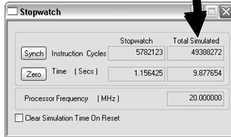
The stopwatch has two pairs of readouts, one tells the **total** simulated clock cycles and the corresponding execution time...<click>
