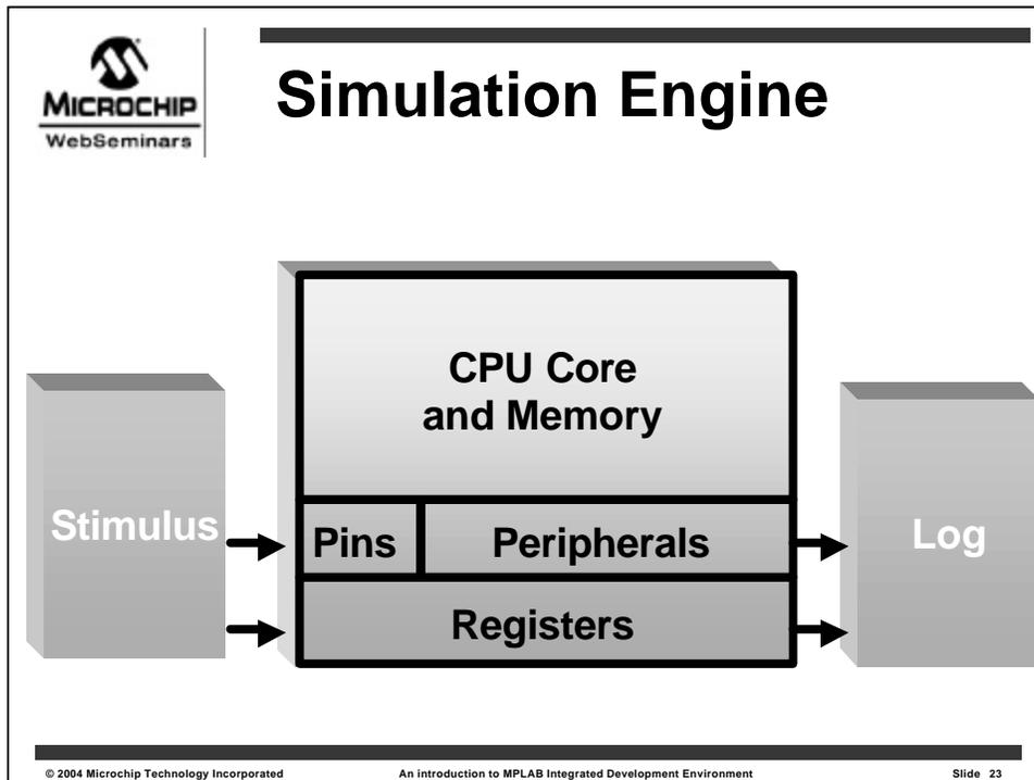
The activity of the simulator can be sent to a **Log file** for later analysis. This is done by using either the **USART** as a communication device for inputs and outputs, or by using the **register log** feature. Both stimulus and logging activity can be driven either by
