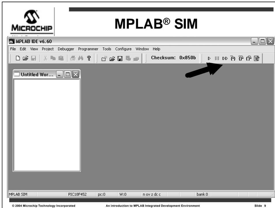
Once a debug engine is selected, the toolbar is appended with some new icons for running, halting, single stepping, and resetting the target.
