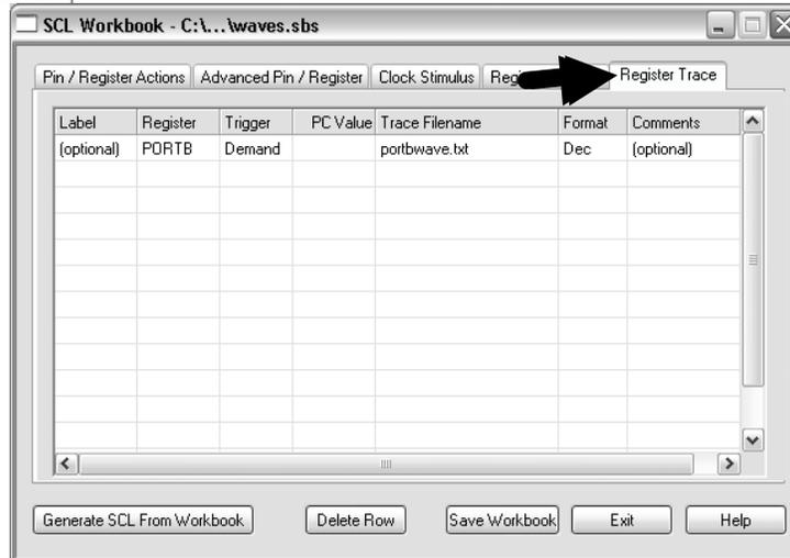
In order to validate that the code is working, we use the **Register Trace** tab of the SCL workbook
