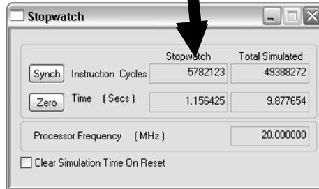
...and the other can be zeroed out, to make a **measurement** from one breakpoint to the next.
