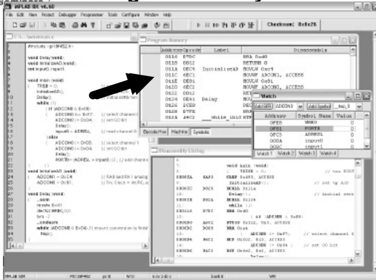
The **Program Memory window** shows the machine code that will be executed by the simulator. Single stepping with this window in focus will allow you to step through each **machine instruction**.
