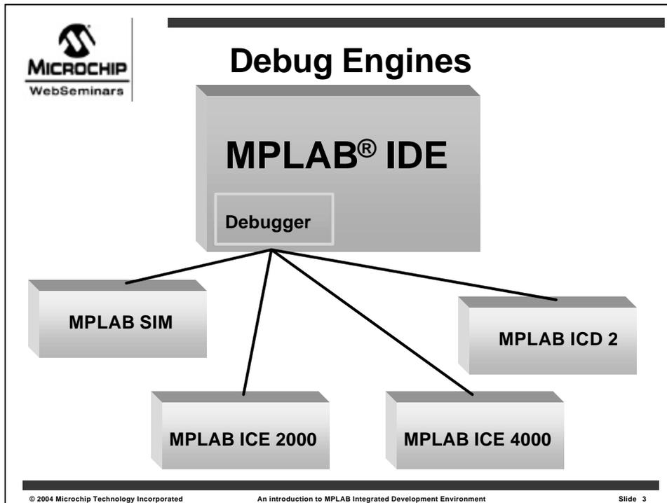
The other debug engines are **hardware** devices, while MPLAB SIM is a **software** program, running on your **PC**.
