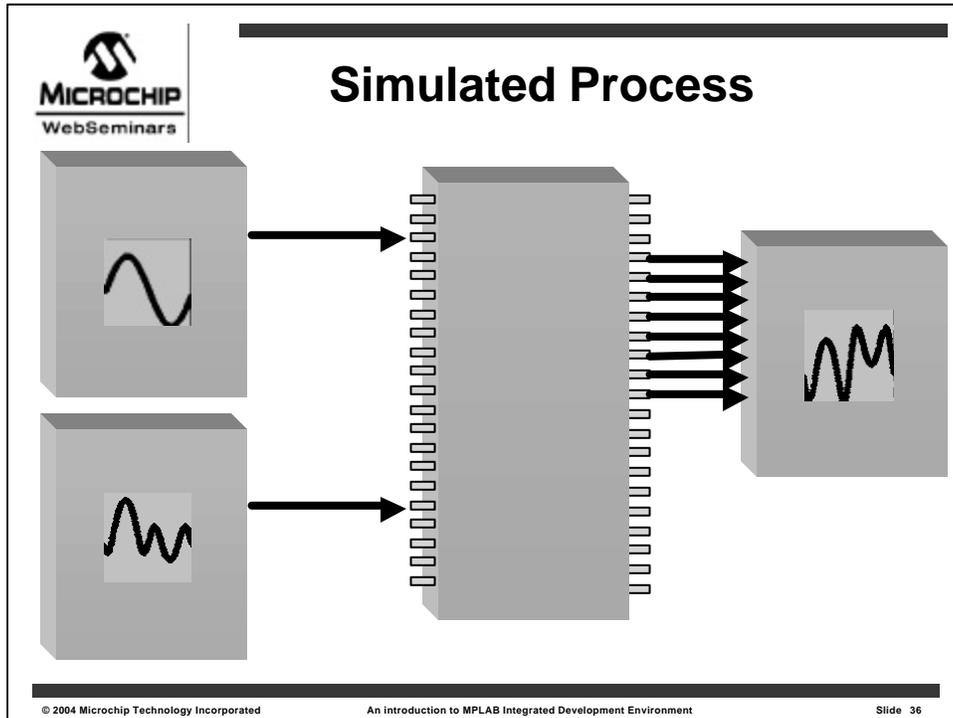
For this next example, **two waveforms** will be **added** together and sent out **PORTB**, possibly to go to a Digital to Analog converter.
