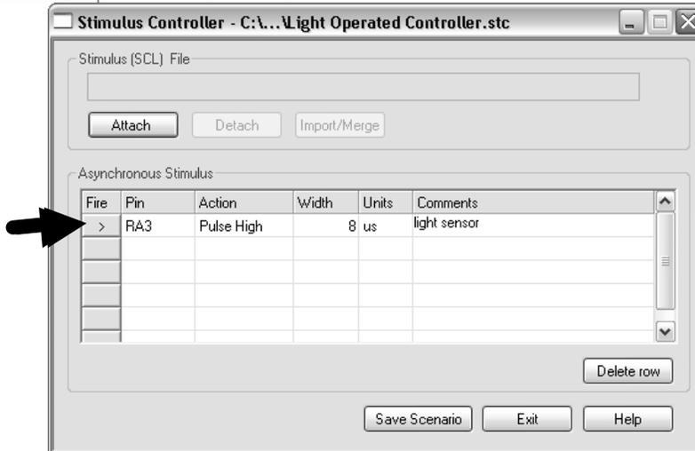
For instance, we could set up a pulse to occur on **PORTA** pin **RA3**.
