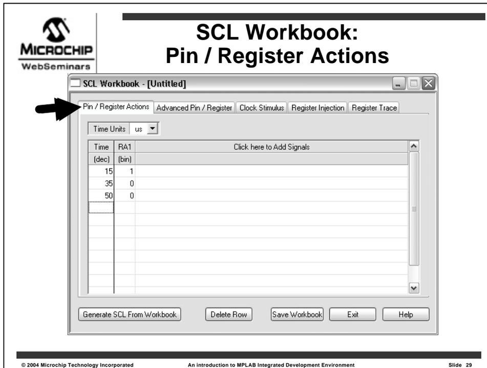
The **first tab** in the SCL Workbook uses a **list of times** and **signals** to be applied to **pins** and **registers**.
