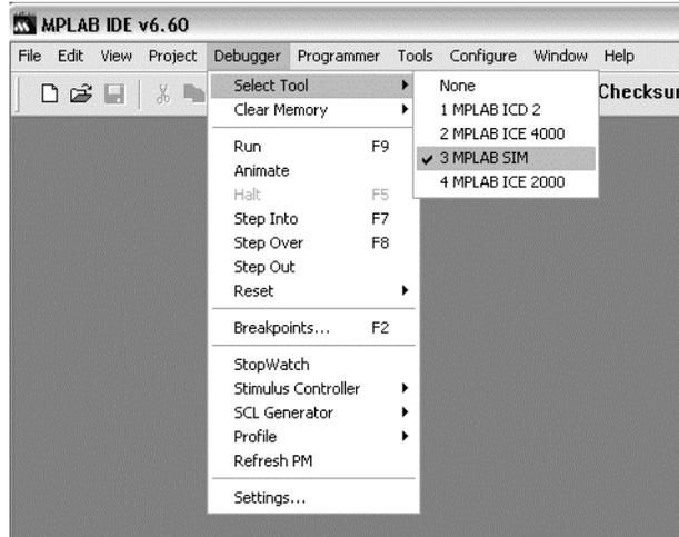
MPLAB SIM is selected as our debug engine from the Debugger menu.
