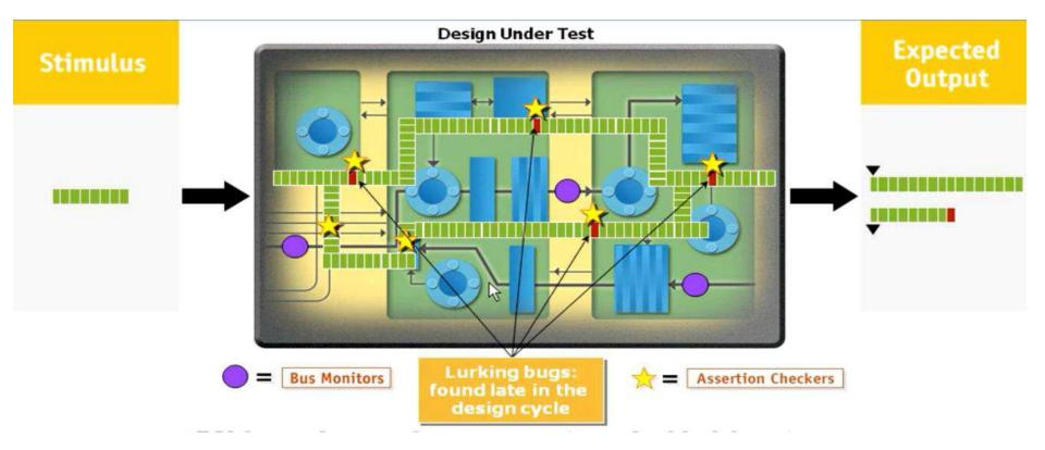
Put assertions at various locations in the design. When an assertion is triggered, you know exactly where it happens. By adding assertions, bad behavior inside the design could be checked and the bugs were observed instantly at their source. Black-box testing vs. White-box testing
