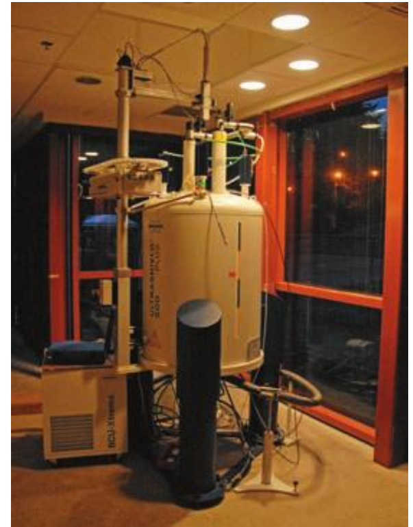
The superconducting magnet of an FTNMR spectrometer
