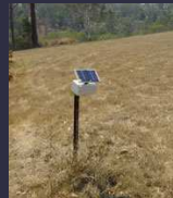
Saltwater intrusion detector (Stephen Brosnan, CSIRO ICT Center)
