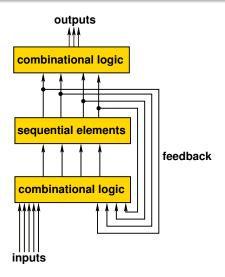
Asynchronous machine block diagram
