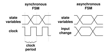
Synchronous vs. asynchronous design
