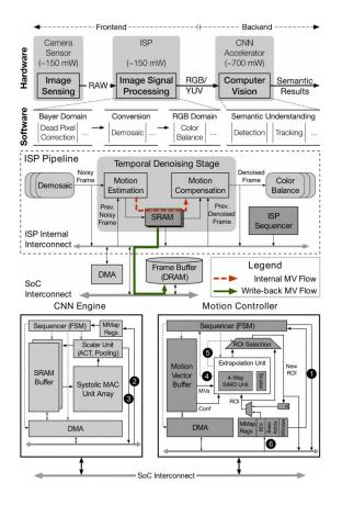
EUPHRATES: Algorithm-SoC Co-Design for Low-Power Mobile Continuous Vision Zhu et. al.
