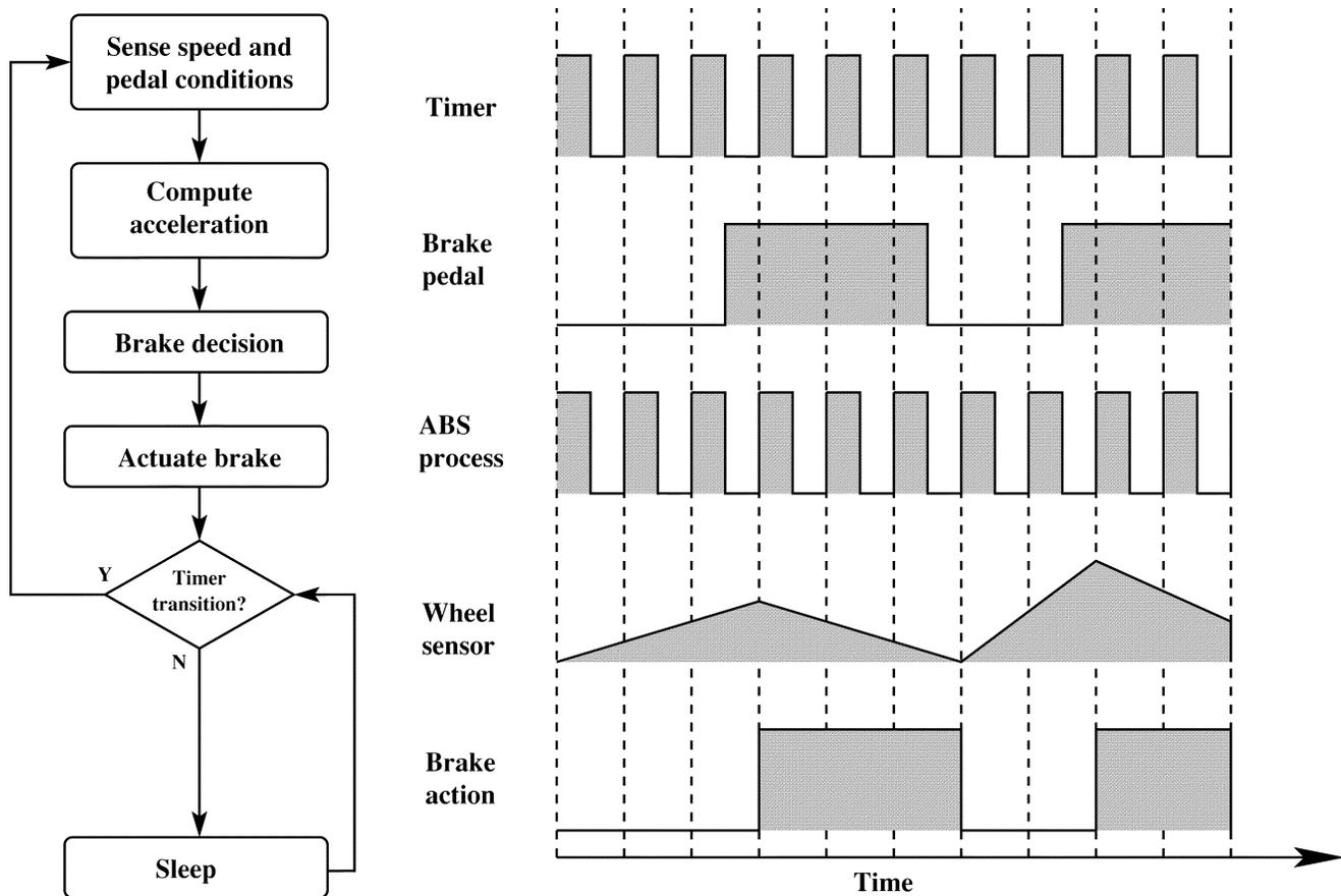
Fig. 1. Straightforward implementation of the ABS example.
