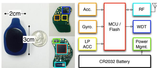
Fig. 2: The Gazelle wearable sensor and system architecture.
