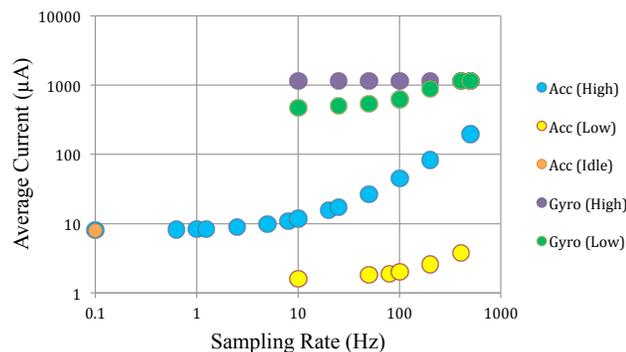
Fig. 1: Power consumption of MEMS IMU sensors: accelerometer, gyroscope, and low-power accelerometer currents are shown across frequency and operational mode.
