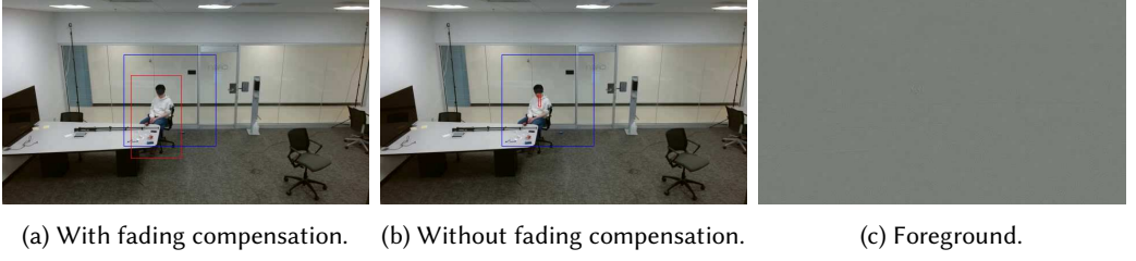
Fig. 10. The UWB box (blue) and final estimate (red) (a) with fading compensation and (b) without fading compensation. When fading happens, pixels in the foreground (c) are almost gray. Without fading compensation, as (b) shows, the final bounding box fails to cover the human figure exposing most privacy-relevant pixels. Fading compensation enables the corrects final bounding box shown in (a).
