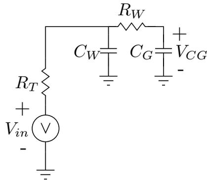
Given that  $V_{in}$  has been 0 V for a very long time, and changes instantly to 2.5 V at  $t = 0$ , derive the expression for  $V_{CG}(t)$ . It is fine to simplify the problem by converting the resistances and capacitances to lump sum values. Please simplify your expression as much as possible.
