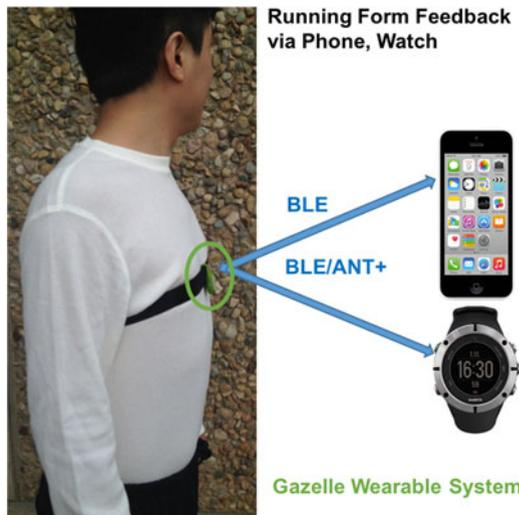
Fig. 3. The example chest worn usage scenario of the Gazelle mobile running analysis system.
